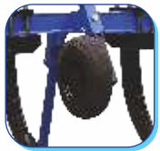
OPTIONAL SUPPORT TYRES SUPPORT & CONTROL DEPTH IN 5 TYNE SUBSOILER
