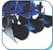
**FURROW OPENER WITH REPLACEABLE WEAR & TEAR POINT AND DEPTH ADJUSTABLE SPIKE**
